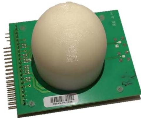
Fig. 22. Fully packaged system with active chip and lens integrated on the PC board for 5G backhaul links.
