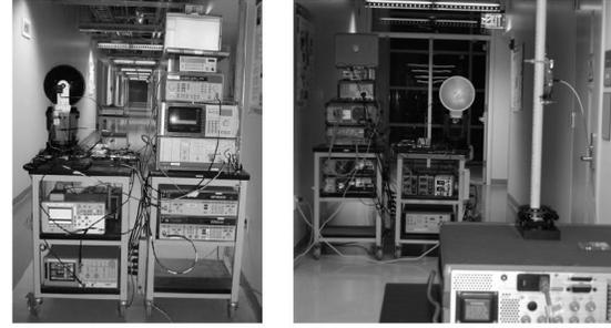
Fig. 6. Indoor radio experiments: the collector system (left) and the view from a sensor (right).
