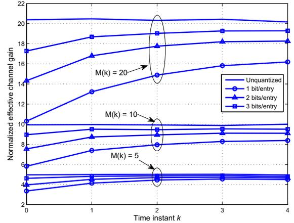
Fig. 4: Plot of  $\bar{\Gamma}_{\text{avg}}$  versus  $k$  in temporally correlated channels for  $v = 10\text{km/h}$  ( $\eta = 0.8721$ ).
