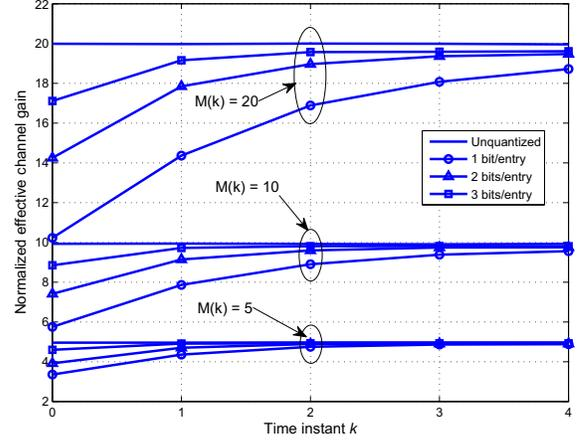
Fig. 3: Plot of  $\bar{\Gamma}_{\text{avg}}$  versus  $k$  in temporally correlated channels for  $v = 3\text{km/h}$  ( $\eta = 0.9881$ ).
