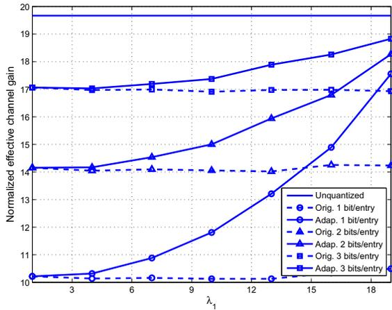
Fig. 6: Plot of  $\bar{\Gamma}_{\text{avg}}$  versus  $\lambda_1$  in spatially correlated channels,  $M(k) = 20$ .
