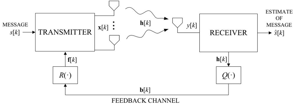
Fig. 1: Multiple-input single-output communications system with feedback channel. The receiver quantizes the current channel realization using NTCQ and sends feedback to the transmitter. The transmitter uses an NTCQ decoder to reconstruct the beamformer.
