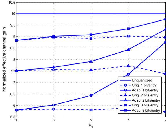
Fig. 5: Plot of  $\bar{\Gamma}_{\text{avg}}$  versus  $\lambda_1$  in spatially correlated channels,  $M(k) = 10$ .
