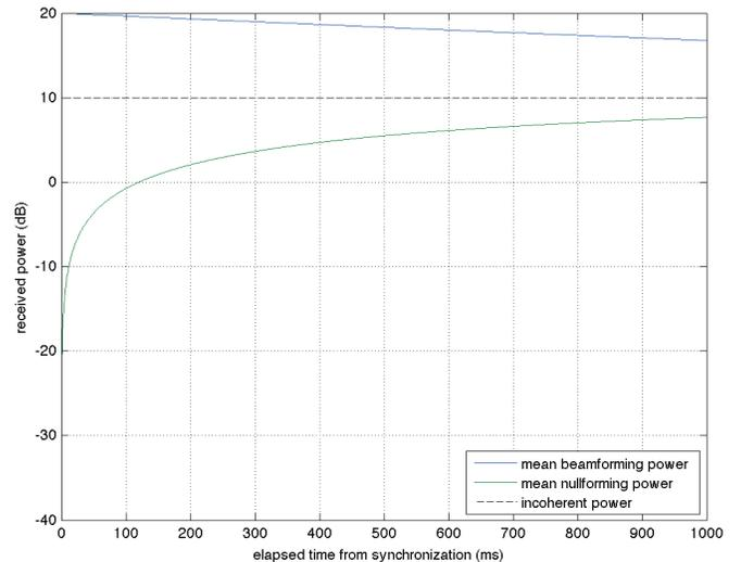
Fig. 8. Nulls deteriorate much faster than beams. The figure shows mean beamforming and nullforming powers as a function of elapsed time from synchronization for 10 cooperating nodes with independently drifting oscillators independently drifting with a standard deviation of 62 ps in one second. The carrier frequency is 2.4 GHz.
