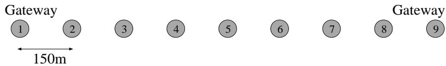
**Figure 4.18:** Nine node line topology: the edge nodes 1 and 9 act as gateway nodes.
