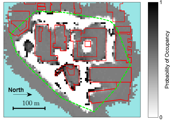
Fig. 6. Horizontal slice (5-10 m above ground level) of generated map covering the eastern portion of the University of California, Santa Barbara campus. The measurement region borders are marked in green, and building contours obtained from OSM are shown in red.
