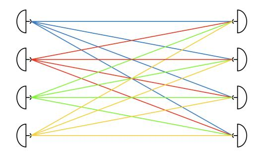
$$\mathbf{H} = \left[ egin{array}{cccccc} h_{11} & h_{12} & h_{13} & h_{14} \ h_{21} & h_{22} & h_{23} & h_{24} \ h_{31} & h_{32} & h_{33} & h_{34} \ h_{41} & h_{42} & h_{43} & h_{44} \end{array}
