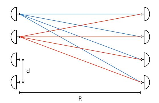
At mm-wave, LOS component dominates. LOS channel is determined by array geometry.
