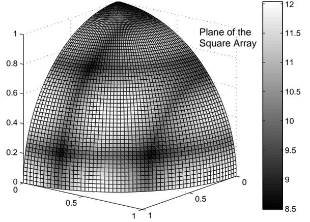
Fig. 3. Beamforming gains (in dB) from a  $4 \times 4$  Row-Column Beamsteerer with linear profile and 4-ary phase quantization. One quadrant of the beampattern is shown on a unit sphere with actual gains (in dB) mapped using gray-scale.
