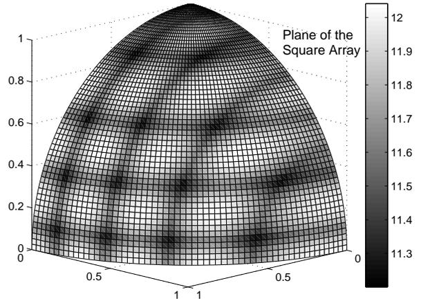
Fig. 4. Beamforming gains (in dB) from a  $4 \times 4$  Row-Column Beamsteerer with linear profile and 8-ary phase quantization. One quadrant of the beampattern is shown on a unit sphere with actual gains (in dB) mapped using gray-scale.
