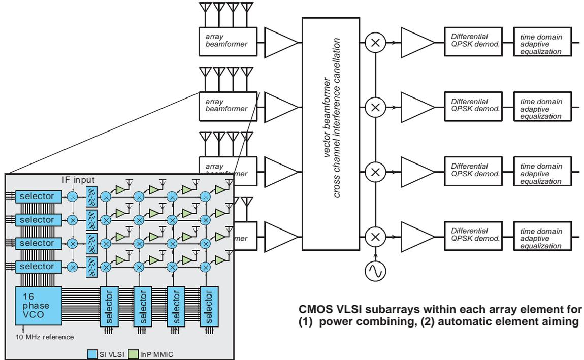
Fig. 5. Detailed description of the row-column beamsteering array VLSI.
