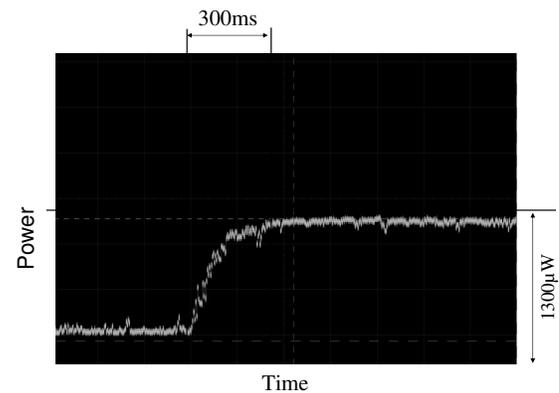
Fig. 10. Received Power Measurement over time
