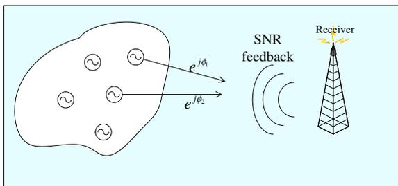
Fig. 1. Phase synchronization using receiver feedback
