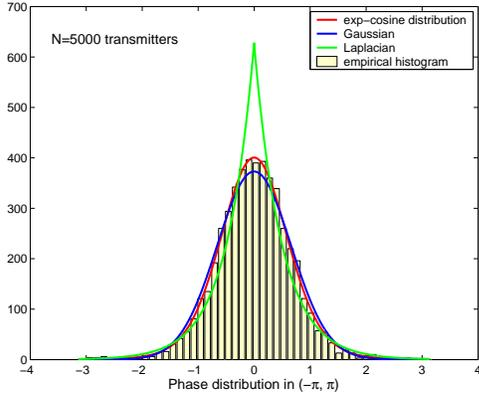
Fig. 5. Histogram of empirically observed phase angles compared with analytically computed distributions
