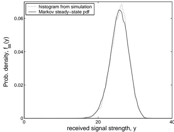
Fig. 11. Distribution of received signal:  $N = 40$ , channel drift  $f_{\Delta}(\Delta_i) \sim \text{uniform}[-\frac{\pi}{25}, \frac{\pi}{25}]$ , phase perturbations  $f_{\delta}(\delta_i) \sim \text{uniform}[-\frac{\pi}{7}, \frac{\pi}{7}]$
