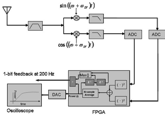
Fig. 8. Block diagram of receiver (BS) prototype
