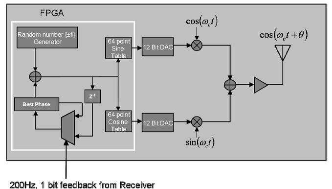
Fig. 7. Block diagram of transmitter prototype
