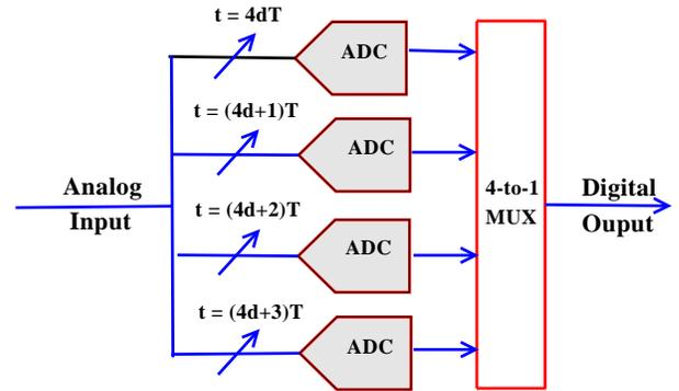
Fig. 1. Ideal time-interleaved ADC with 4 sub-ADCs. The sampling instants ( $d = \text{integer}$ ,  $T_o = \text{sampling period}$ ) of the sub-ADCs are staggered such that each sub-ADC operates at one-fourth of the net sampling rate of the TI-ADC
