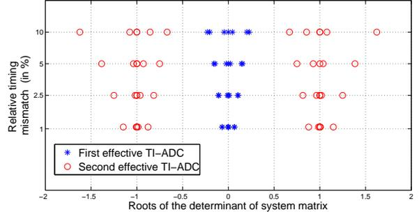
Fig. 3. Zeros of the determinants of the matrices  $B$  and  $C$  (corresponding to the two effective TI-ADCs in 2x oversampling) as a function of relative timing mismatch. The zeros are all real and there are no zeros of  $\det C$  beyond the depicted range. We ignored any common zeros at  $z = 0$ .
