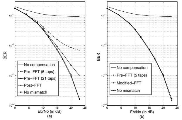
Fig. 4. BER in a 64-QAM, 128-subcarrier OFDM system employing a sloppy TI-ADC with 10% timing mismatch. For the left subfigure (a), Nyquist rate sampling is performed and the TI-ADC interleaving factor  $L$  is 8. On the other hand, we assume two times oversampling and  $L = 32$  in the right subfigure (b). The Modified-FFT approach corresponds to an OFDM-specific mismatch compensation approach given in [14].
