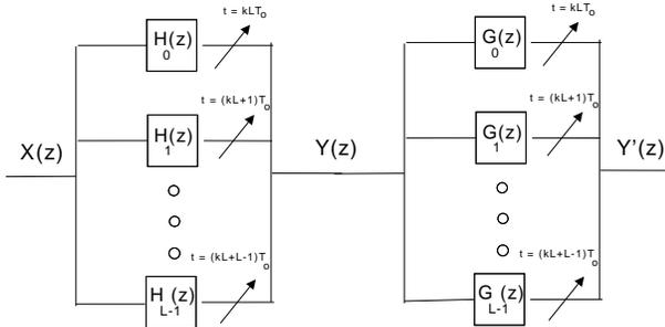
Fig. 2. Linear model for mismatch in a TI-ADC and zero-forcing based mismatch compensation ( $k$ =integer,  $T_o$ =sampling period). All symbols indicate discrete streams at the symbol rate  $T_o^{-1}$ .
