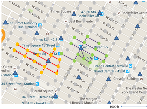
Fig. 8: Clusters in a typical mesh backhaul in an urban environment mapped from part of New York City. Triangles and circles represent gateway non-gateway nodes respectively.
