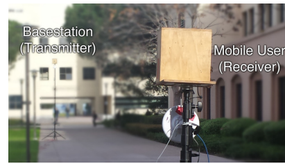
Figure 4: Our 60GHz phased array testbed emulating picocells.
